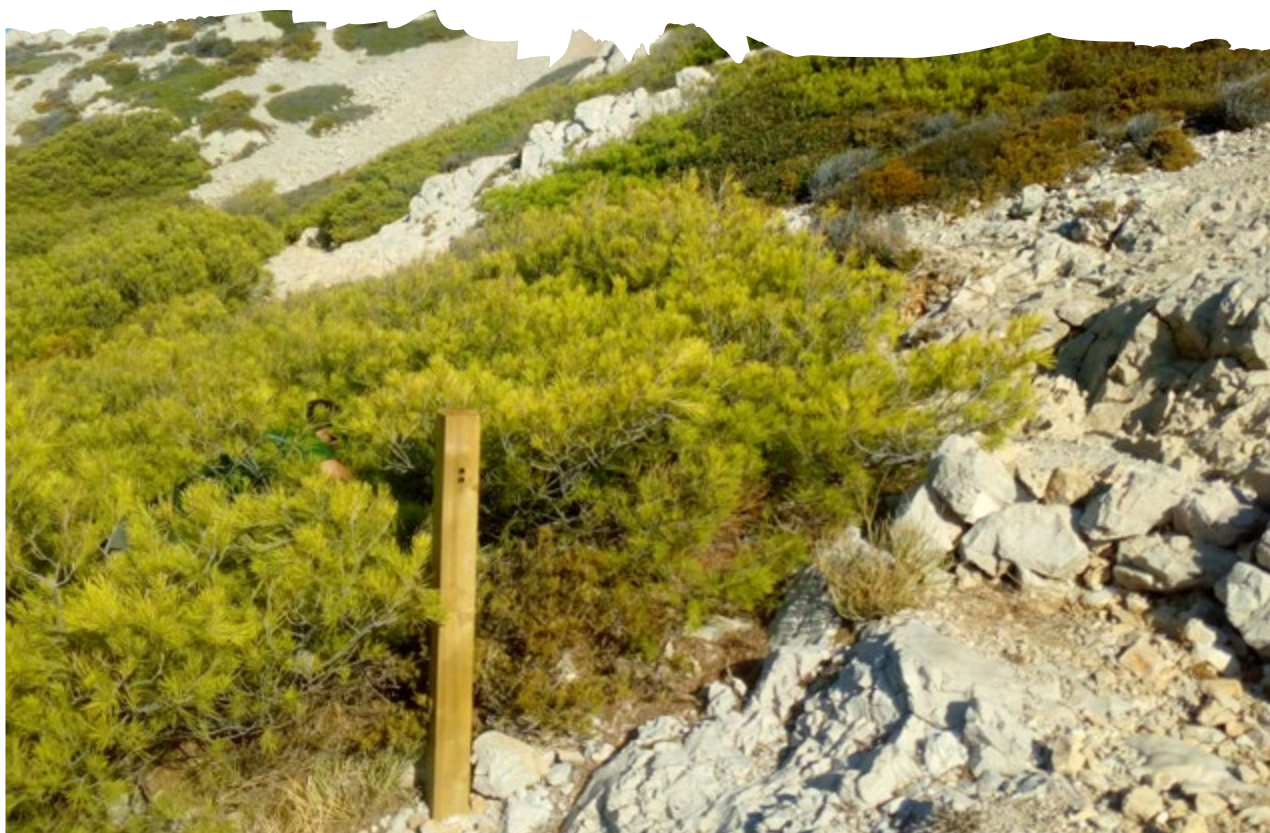
PYRO eco-counter camouflaged in a wooden post at the entrance to a footpath closed off by rocks, Callelongue-Marseilleveyre sector
